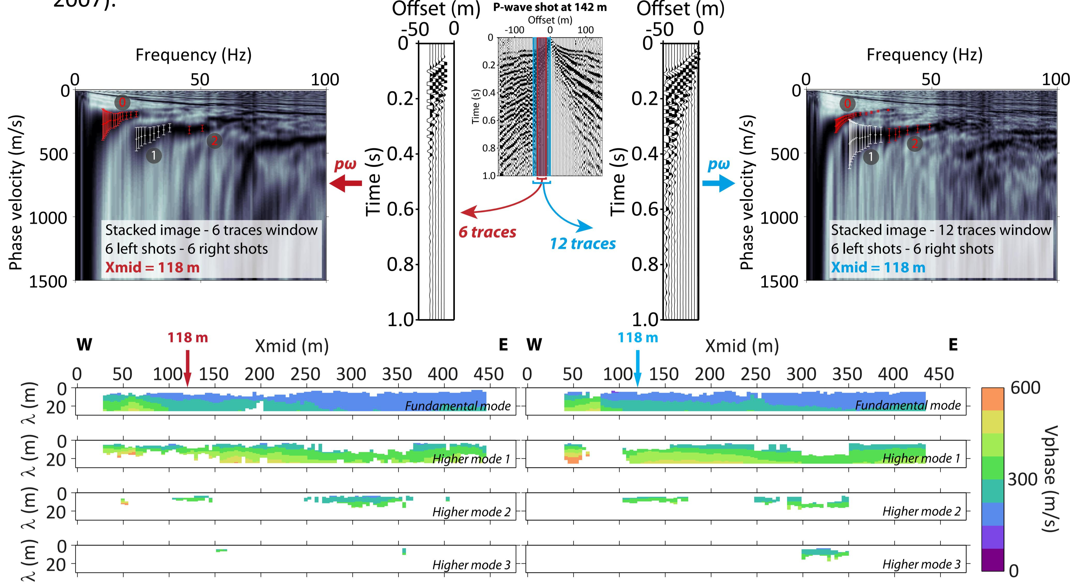
**Dispersion inversion:** 1D inversion using a Neighborhood Algorithm (Wathelet *et al.*, 2004) at each  $X_{mid}$ ; average  $V_s$  model build from models fitting within the error bars; 2D  $V_{s^{SWP}}$  section reconstruction (Strobbia *et al.*, 2011) with no lateral constraint.
