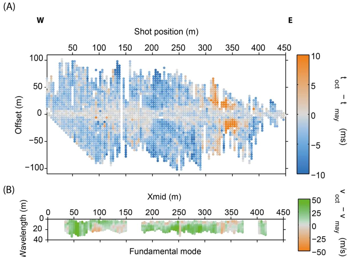
**Figure 2** (A) P-wave picked first arrival time absolute differences, represented as a function of the offset and source positions. (B) Absolute differences of picked Rayleigh-wave phase velocity dispersion curves. Only the fundamental propagation mode is presented as a function of the wavelength and the spread mid-point ( $X_{mid}$ ). In both cases, the differences are calculated between October 2011 and May 2012.
