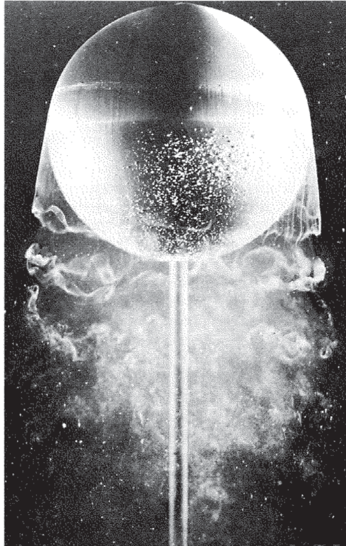
Fig. B6.1 Visualization of flow around a sphere to show the onset of turbulent flow separation. (From van Dyke, 1982.)
